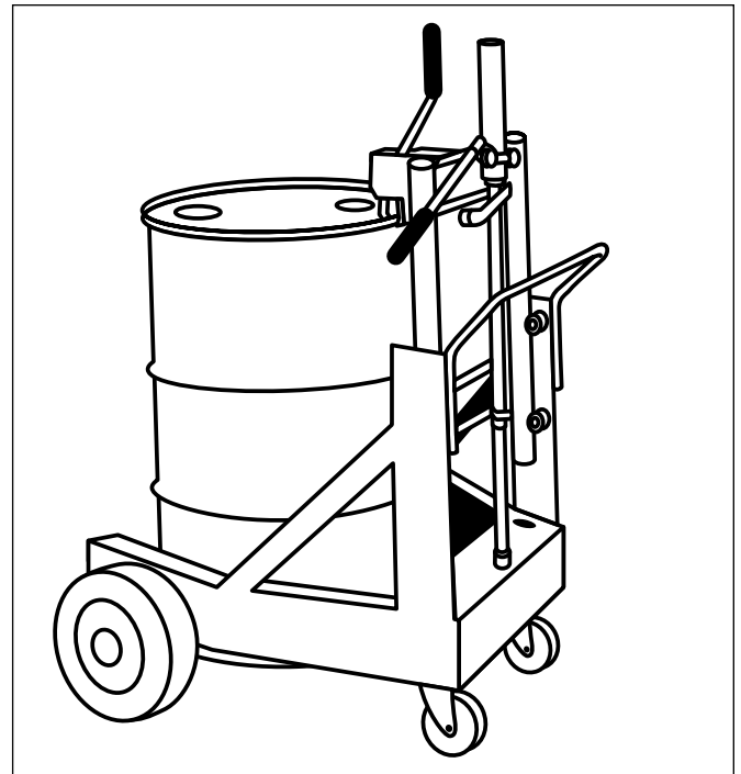
Fig. 5—Manual Drum Handler Hand-operated hydraulic systems clamp the drum, then lift it for transportation.
