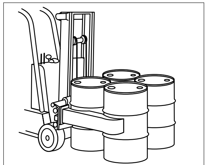
Fig. 4—Fork Lift Adapters for Handling Drums Various types of adapters are available which can be installed on forklift trucks for handling drums. Models are available to handle from one to four drums at a time. Some models can be used to invert the drums.
